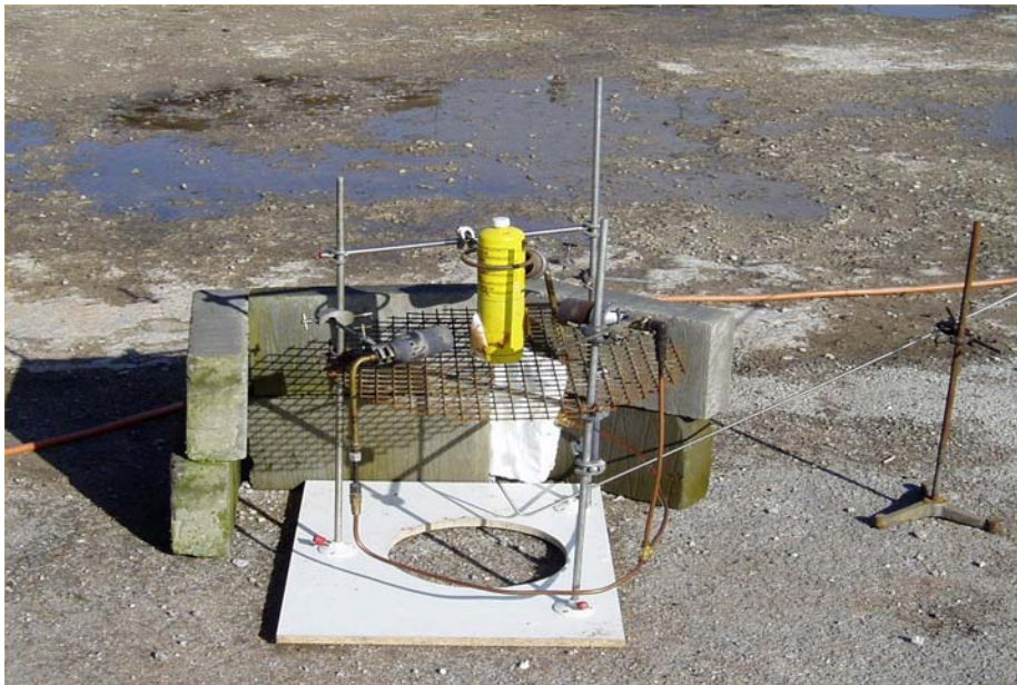
Figure 5: Burner assembly for Test Series D.
